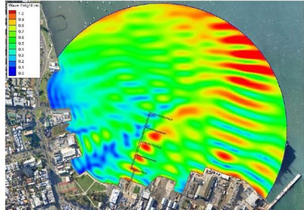
Figure 5 Model output showing wave height contours for 17s,  $10^\circ N$ , existing marina. Note contours are relative to a 1m incident wave height for ease of comparison of amplification factors.
