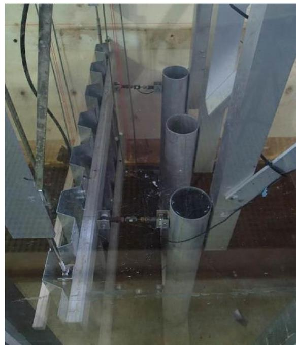
Figure 9 Geometrically similar partial depth wave screen model in 0.9m wide wave flume. Note the load cells placed between the wall and piles. Gap below wall not visible.
