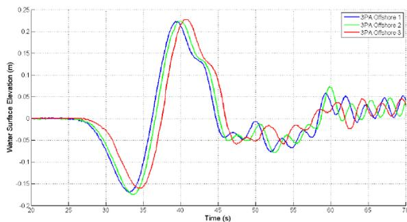
Figure 10 Wave probe record of 19.9 second Bernoulli wave test. Note the strong initial draw-down and sharp surge.
