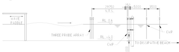
Figure 7 Wave flume set-up
