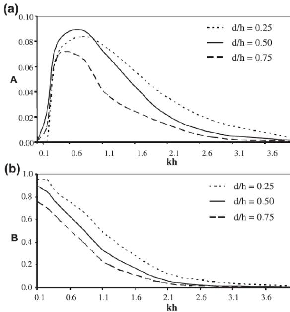
Figure 4 Values of A and B for determining  $\alpha$  (Source [3])
