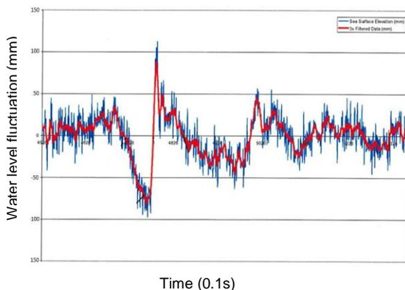
Figure 3: Characteristic Bernoulli wave in Hobsons Bay resulting from ships transiting the nearby Williamstown Channel (Source: [6]).
