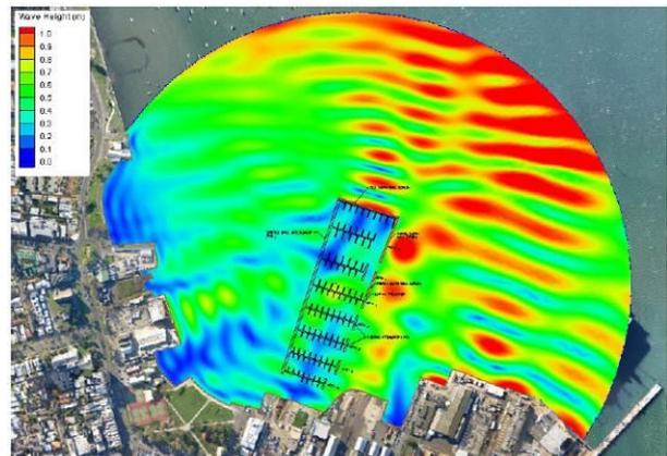
Figure 6 Model output showing wave height contours for 17s,  $10^\circ N$ , proposed marina.
