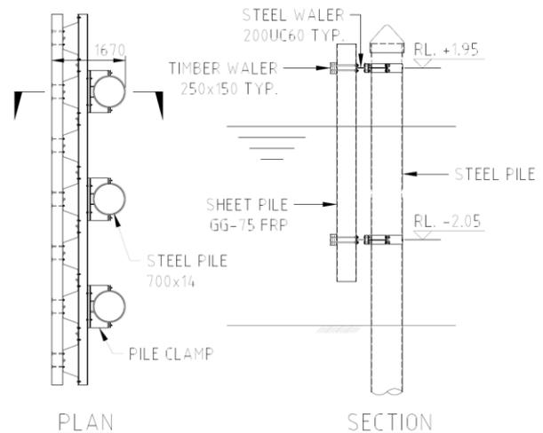
Figure 8 Partial depth wave screen to be tested by wave physical modelling
