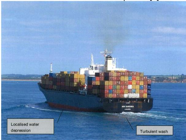
Figure 2 Bernoulli wave evident on side of tanker transiting the entrance to Port Phillip Bay (Source: [6]).
